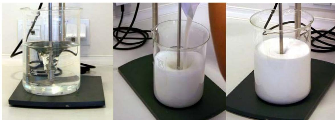
**Figure 1. a:** Propeller stirrer properly positioned in mixing vessel. **b:** Addition of Aquarius™ film coating system powder to the solvent solution. **c:** Mixing for 60 minutes.
