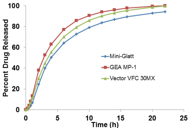
**Figure 8 Dissolution Results Obtained When Coating Venlafaxine Pellets with an EC Coating Containing a Pore Former (EC:HPC ratio 3.5:1) on Various Processing Scales**
