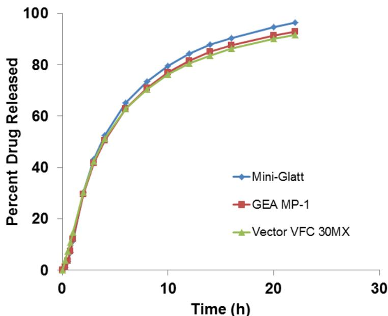
**Figure 7. Dissolution Results Obtained When Coating Venlafaxine Pellets with an EC Coating (No Pore Former) on Various Processing Scales**
