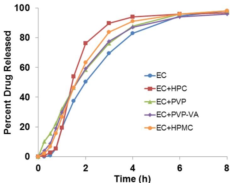
**Figure 1. Influence of Pore-forming Agents (EC-PFA Ratio 3.5:1) on Drug Release from Venlafaxine Pellets Coated with Ethylcellulose Coatings (10% weight gain)**
