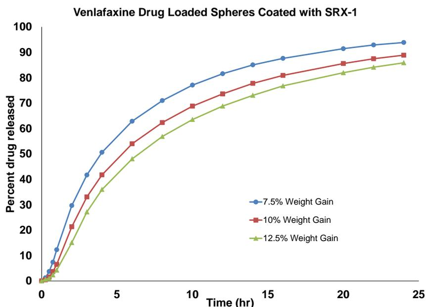
**Figure 5. Initial Dissolution Results Obtained When Coating Venlafaxine Pellets with an EC Coating (No Pore Former) Using the Mini-Glatt**
