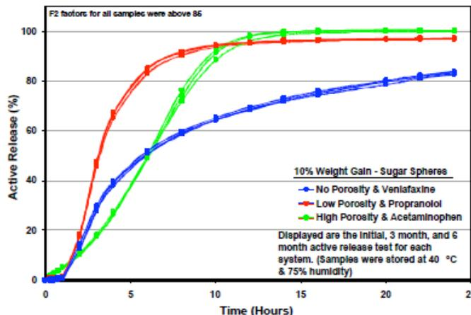
**Figure 3:** Release and Stability of Drug layered sugar spheres coated with Aquarius SRX
