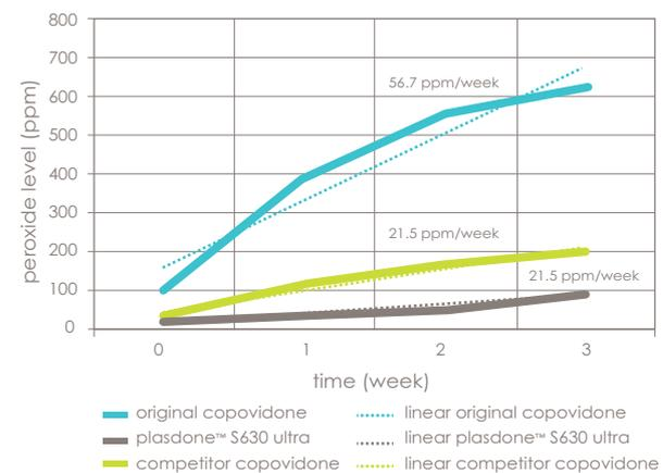
As seen in Figures 6 and 7, extrudates prepared with Plasdone™ S630 Ultra copovidone demonstrate a lower yellowness index and significantly lower peroxide levels compared to those prepared with original copovidone at various extrusion temperatures.
