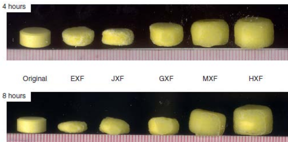
Figure 4 Effect of Fine Particle Klucel™ HPC MW on Erosion and Swelling Behavior Nifedipine Matrix Tablets Subjected to Dissolution Testing for 4 and 8 Hours Formulation: 20% Nifedipine, 30% HPC, 49.5% MCC, 0.5% Mag Stearate (Ruler shows 1mm spacing).
