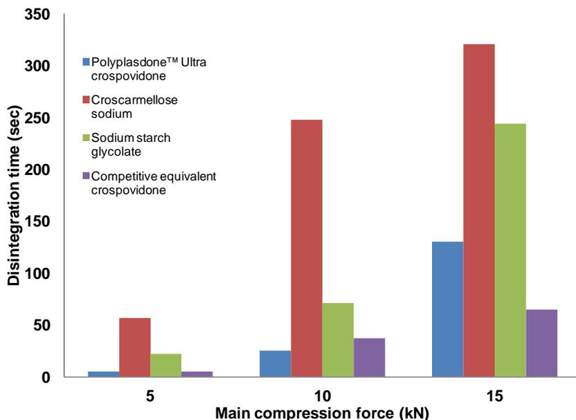
Figure 6. Effect of compression force on disintegration time of fenofibrate ODTs
