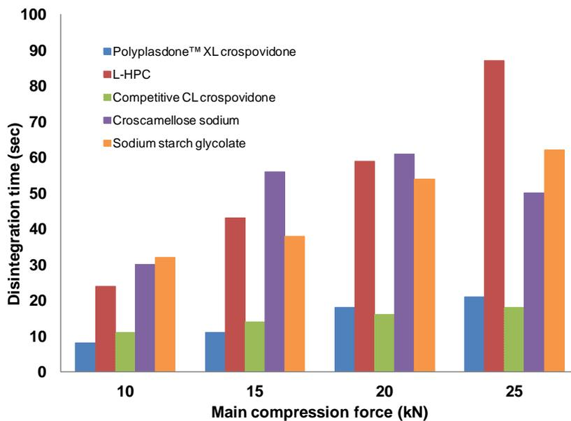
Figure 3. Effect of compression force on disintegration time of acetaminophen ODTs
