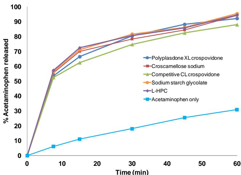
Figure 4. Dissolution profile of acetaminophen ODT in pH 5.8 phosphate buffer
