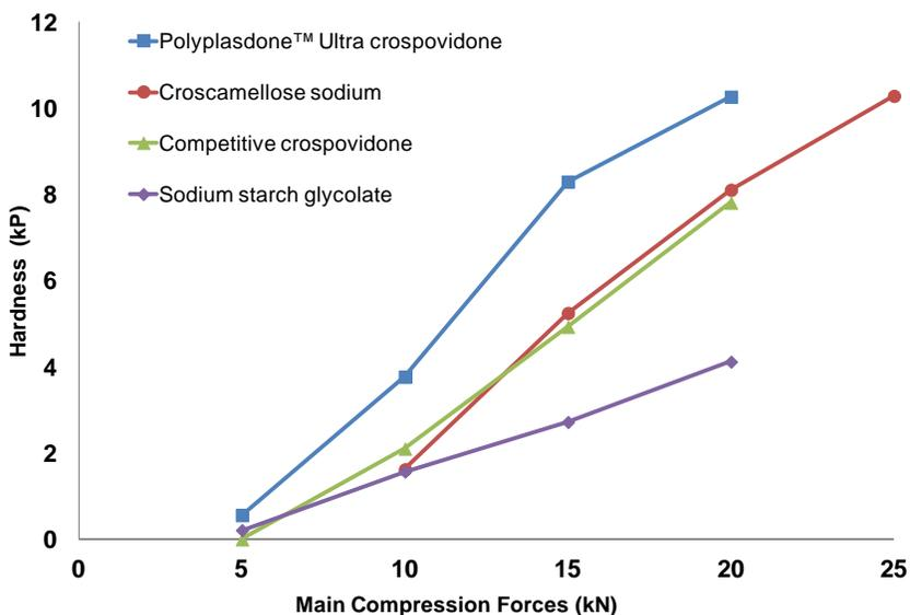
Figure 5. Effect of compression force on hardness of fenofibrate ODTs
