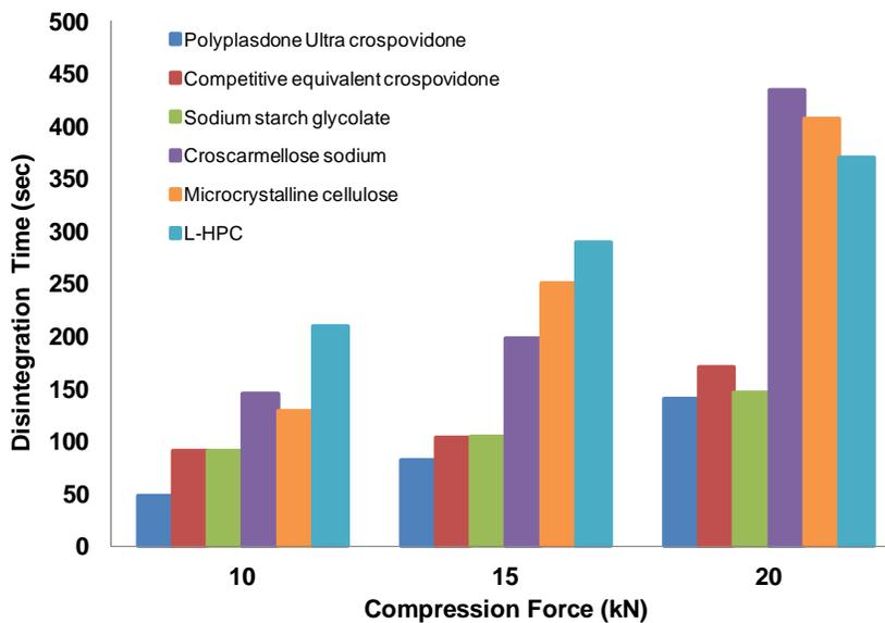
Figure 4. Disintegration time of IR ranitidine HCl tablets
