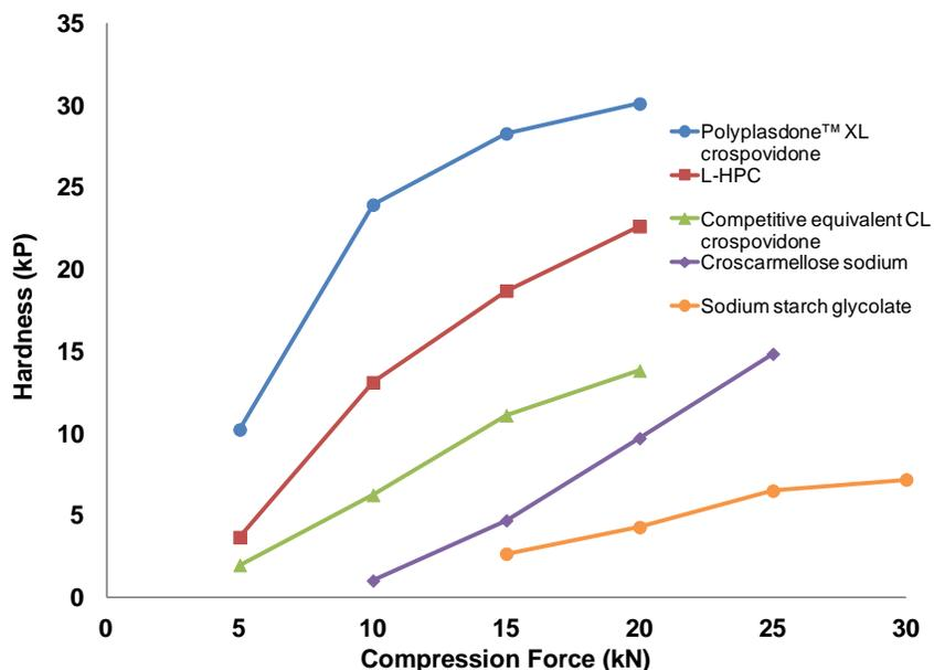
Figure 2. Pure polymer compaction comparison of superdisintegrants
