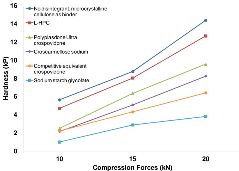
Figure 3. Effect of compression force on hardness of IR ranitidine HCl tablets
