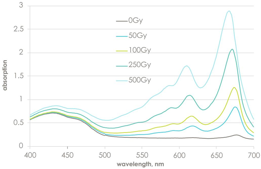
figure 3. spectra of Gafchromic™ HD-V2 as a function of absorbed doses
