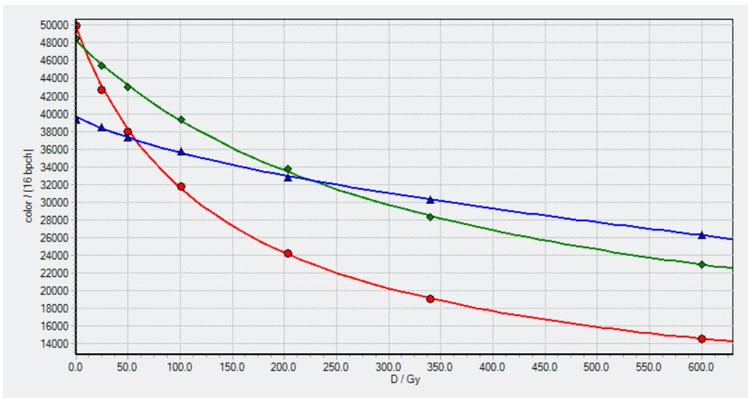
figure 4. response of Gafchromic™ HD-V2 in all color channels
