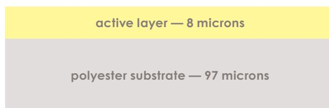
figure 1. configuration of Gafchromic™ HD-V2 dosimetry film
