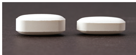
Figure 1. Lower binder use levels enable approximately 20% size reduction in final tablet size
