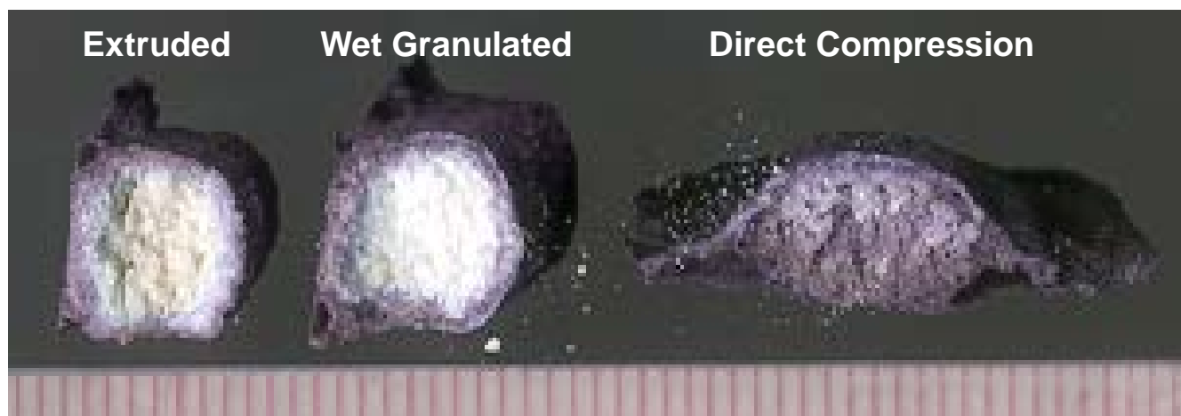
Figure 5. Media uptake of Metformin HCl tablets. The tablets were submersed in a blue dye solution for 30 minutes and then dried overnight. Pictures of the cross sectional surfaces were then taken.
