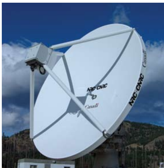
Composites beat out metals for lighter, stiffer, high-performance radar telescope reflector dishes.
