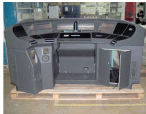
FRP provides high durability and minimal assembly requirements in engine consoles.
