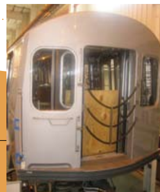
Subway car end caps fabricated by Fênix for NY Subway
