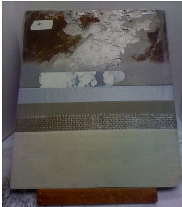
Figure 5. Heavily Pitted Duplex Stainless Steel with Epoxy Vinyl Ester Flake Glass Repair Lining – Courtesy of Blome International
