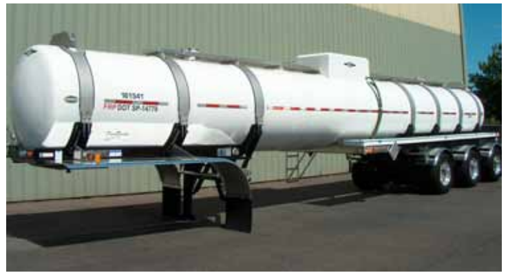
Corrosion Companies' composite cargo tanker.
