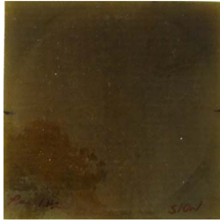
FIGURE 9 – Br NEVER FRP laminate with carbon and c-glass veil exposed to test solution for 24 weeks and 1 hour at 204°C
