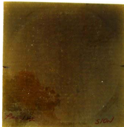
FIGURE 8 – Br NEVER FRP laminate with carbon and c-glass veil exposed to test solution for 24 weeks and 1 hour at 182°C
