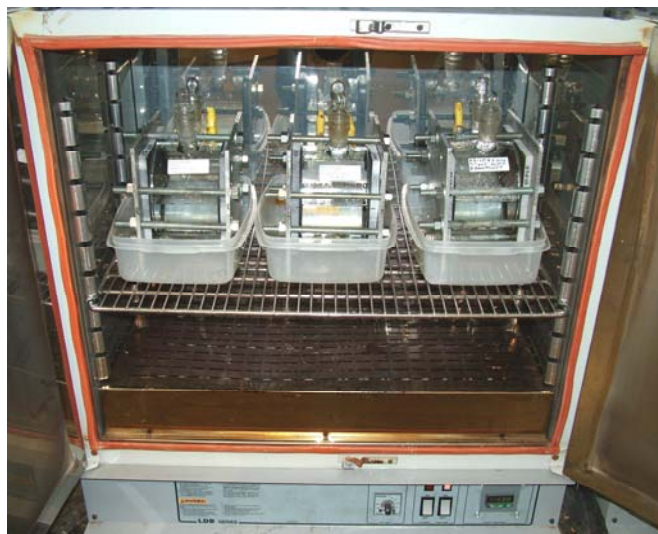
FIGURE 2 - Atlas test cell placement in oven.
