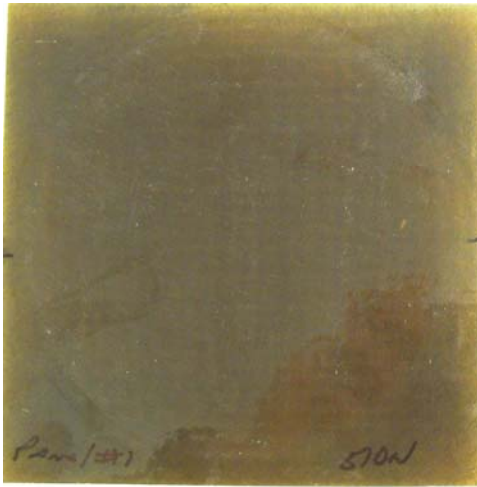
FIGURE 11 – Br NEVER FRP laminate with carbon and c-glass veil exposed to test solution for 36 weeks and 1 hour at 182°C
