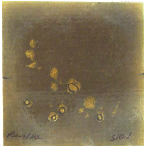
FIGURE 12 – Br NEVER FRP laminate with carbon and c-glass veil exposed to test solution for 36 weeks and 1 hour at 204°C
