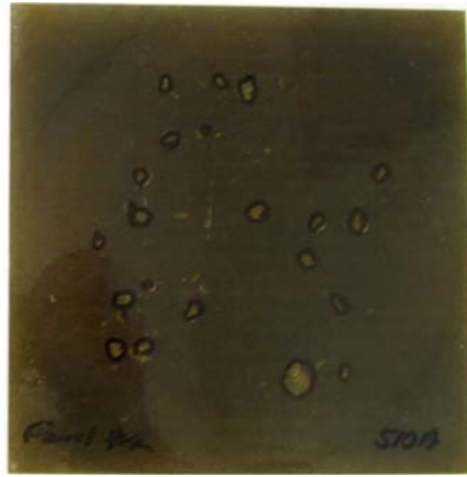
FIGURE 7 – Br EVER FRP laminate with a carbon and c-glass veil exposed to test solution for 12 weeks and 1 hour at 204°C
