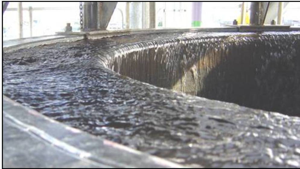
Figure 4. FRP Weir Bowl and creation of the protective liquid curtain on the interior of the primary DynaWave ® inlet barrel.
