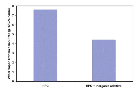
Figure 2b Effect of including and inorganic platy additive on moisture uptake of coated copper sulfate tablets
