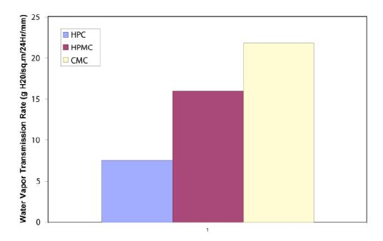
Figure 1b Effect of polymer hydrophilicity on moisture uptake of copper sulfate tablets coated with polymer only. HPMC is more hydrophilic than HPC.
