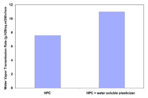
Figure 4b Effect of water soluble plasticizer on moisture uptake of coated copper sulfate tablets
