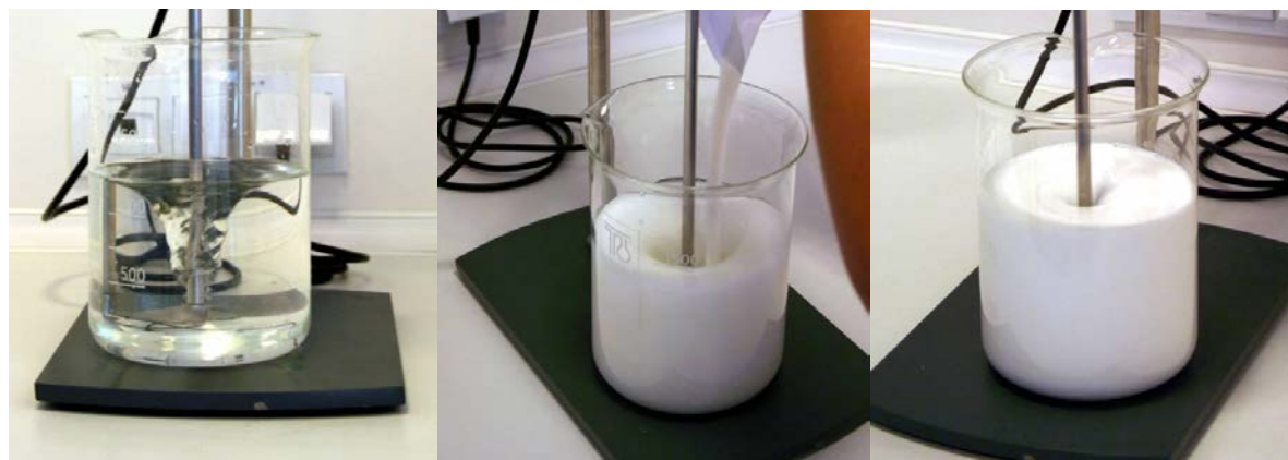
Figure 1. a: Propeller stirrer properly positioned in mixing vessel. b: Addition of Aquarius film coating system powder to the water. c: Mixing for 60 minutes.
